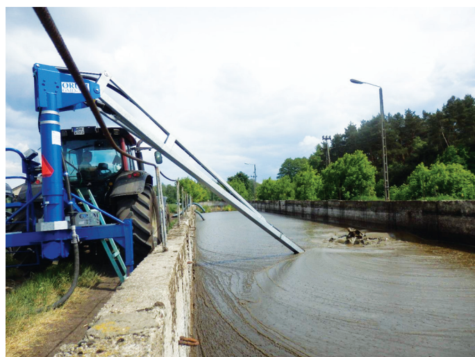
Fig. 3. Dosing of sulfuric acid to the slurry mixer arm
