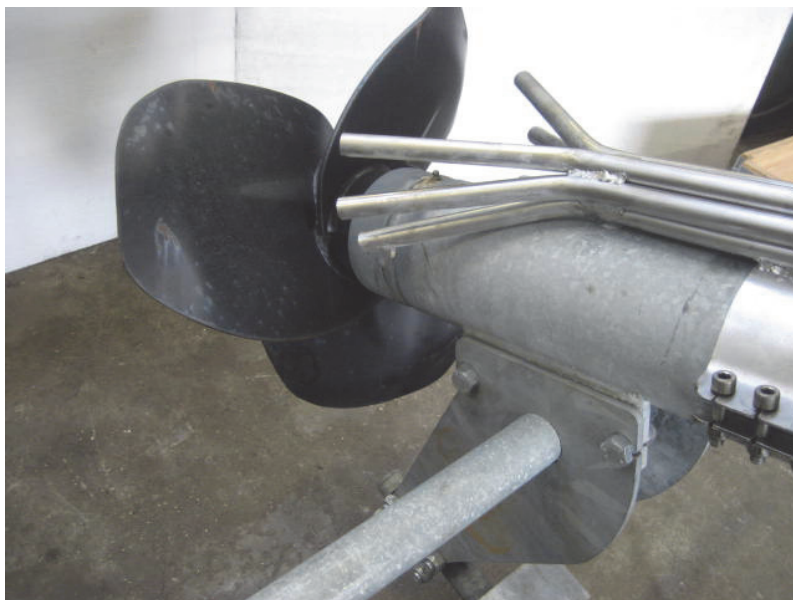
Fig. 5 Detailed view on acid discharge system of ORUM Co.– construction of “in storage” unit (Orum Semden’s)
